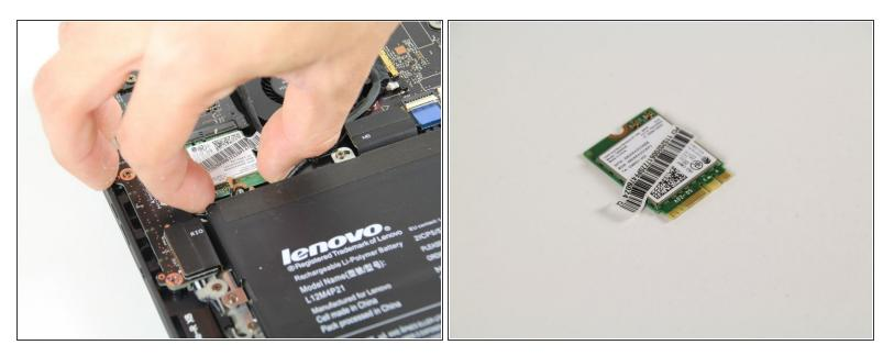
• Slide the wireless module towards the battery and lift out of the laptop.
