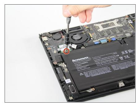
Remove the one 1/16" screw using a Phillips #00 screwdriver.
