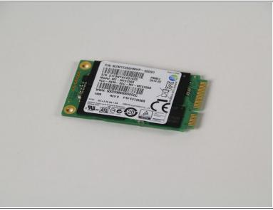
• To remove the solid state drive, gently slide it away from the battery and towards the hinges.
