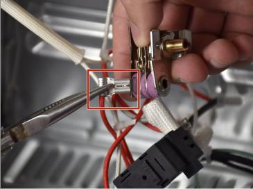
Press down the metal tab on the oven heat control connector using needle nose pliers and pull outwards to remove the connector.
