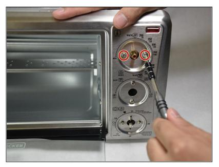
Remove the two 5.5mm screws, that are holding the oven controls to the face, using a #2 Phillips head screwdriver.
