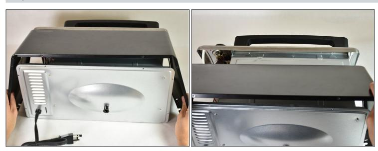
Remove the back cover by gently pulling the sides of the cover apart from the rest of the oven.
