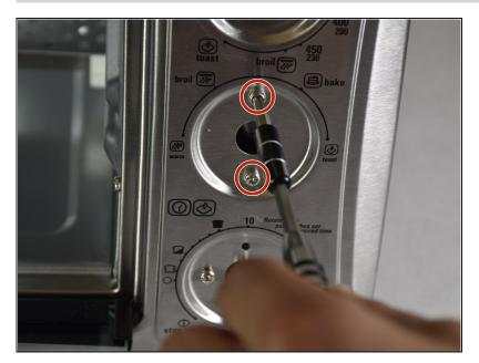
Remove the two 7.5mm screws, that hold the toaster controls to the face, using a #2 Phillips head screwdriver.
