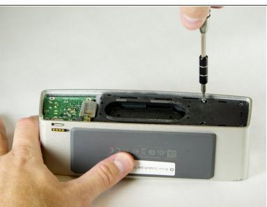
Remove the four 15.0 mm screws on the left and the four 9.0 mm screws on the right using the T8
