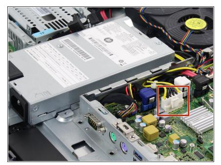
Disconnect the power supply's black and yellow cable from the motherboard.
