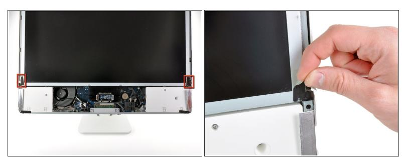
• Peel the two highlighted EMI shield tabs off the frame of the LCD.
