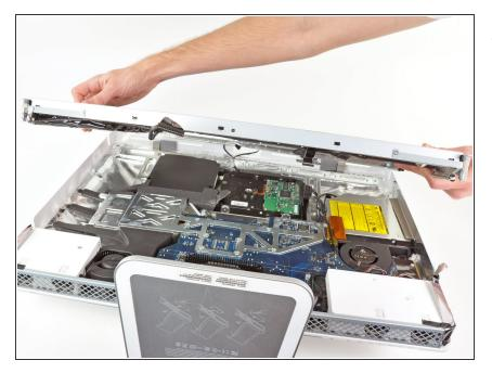
• Remove the display assembly from the iMac.
