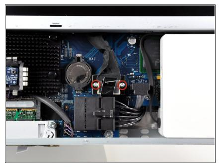
Remove the two T6 Torx screws securing the display data cable to the logic board.
