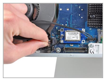
• Pull the CPU fan connector toward the left edge of the iMac to disconnect it from the logic board.
