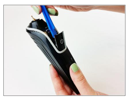
Apply pressure to pry off the power button.
