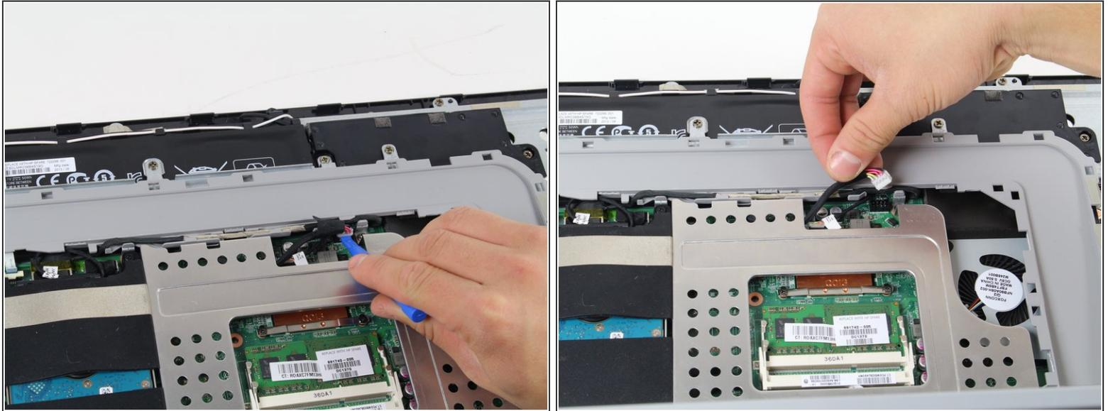
**!** Before working on any of the internal components of the computer, make sure the battery is disconnected so there's no power running through the device.
