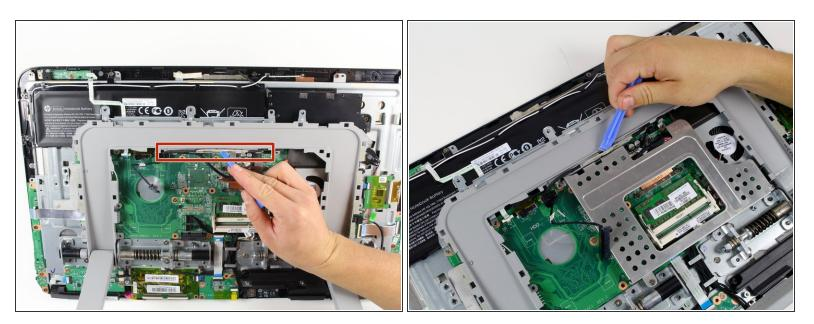
• Gently remove wires from around the stand recess with the plastic opening tool.
