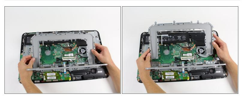
Remove the stand recess by moving it towards yourself, rotating it about the hinge and then taking it out of the computer.
