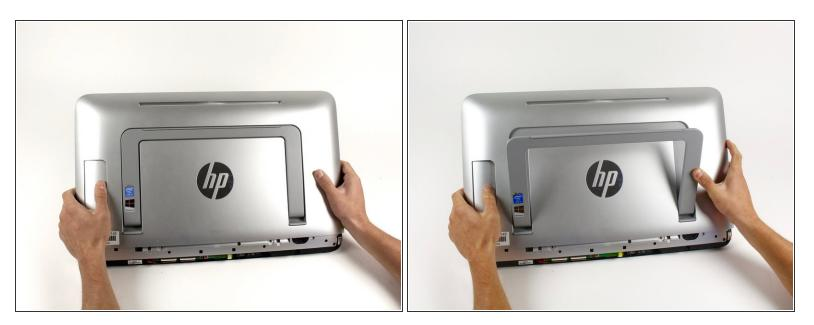
Release the stand by pressing the large button on the left so that it is easier to take the back case off.
