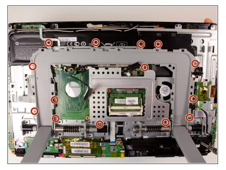
Remove the fourteen 6.35 mm PH#0 screws around the stand recess and metal cage.
