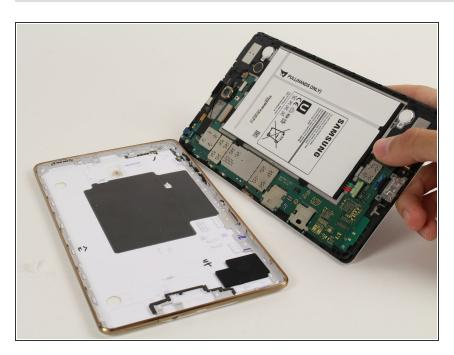
Remove the back cover after the entire rim is disconnected.
