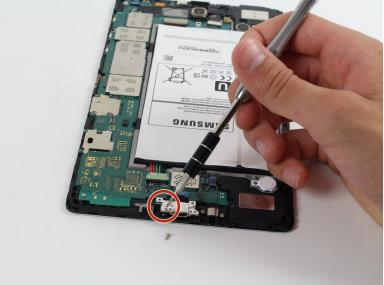
• Remove the two 4 mm Phillips #000 screws securing the micro USB port.
