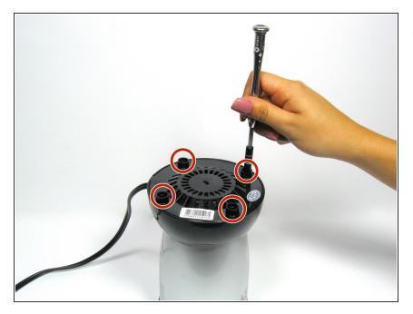
Remove the four 14.0 mm Phillips head screws in the feet of the base of the Magic Bullet using the Phillips #1 screwdriver.
