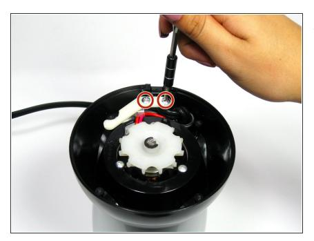
Remove the two 13.0 mm Phillips head screws from the white plastic cable guide using a Phillips #1 screwdriver.
