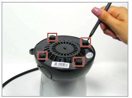
Remove the four rubber pegs from the feet on the base of the Magic Bullet using the spudger.
