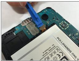
Using the plastic opening tool, gently pry the chip connections away from the motherboard.
