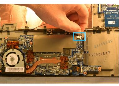
Gently pull the motherboard out by pulling from the right side of the board and flip it so that the motherboard now sits where the battery was and the underside is now visible.
