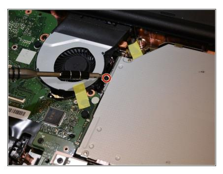
Using a #0 Phillips screw driver, remove the (5mm) black screw to the left of the CD Drive and to the right of the cooling fan.
