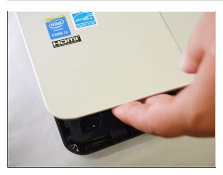
You can now fully remove the keyboard and front panel to gain access to the inside of the laptop.
