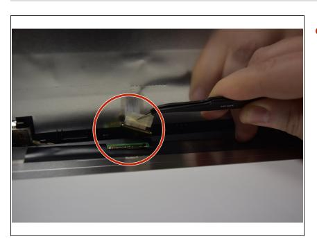
Take the metal angled tweezers to detach the connector from the back of the screen.
