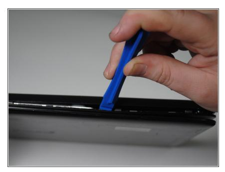
Using a plastic opening tool, work around the Chromebook separating the plastic case at the seam.
