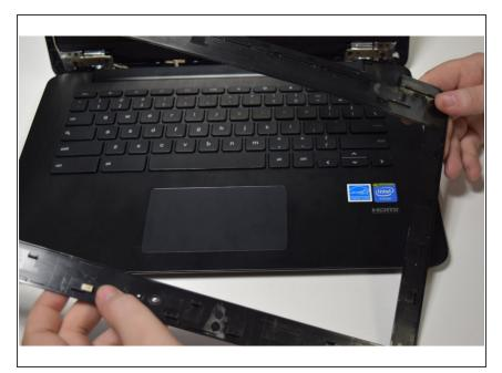
Completely remove the inner screen liner and set aside.
