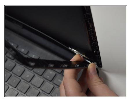
Pop the inner screen liner using your fingers, gently, until completely separated from the screen.
