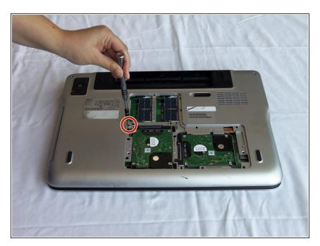
Unscrew the screw holding the optical drive with a Phillips screwdriver.
