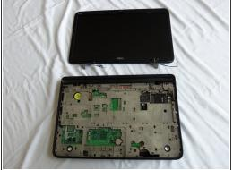
Hold the plastic edge of the display firmly and lift to remove the display.
