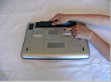
Slide the tab below the battery to the left and hold the tab in place.
