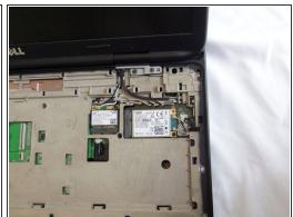
Insert the pointy side of the spudger below the golden connector of the white cable on the WLAN card and lift to detach.
