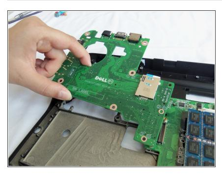
Lift and remove the Wi-Fi circuit board.
