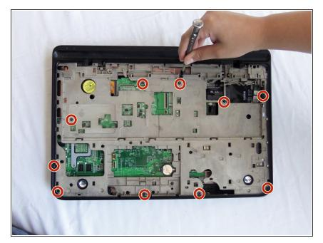
Unscrew the ten 8mm screws from the grey inner casing with a Phillips screwdriver.
