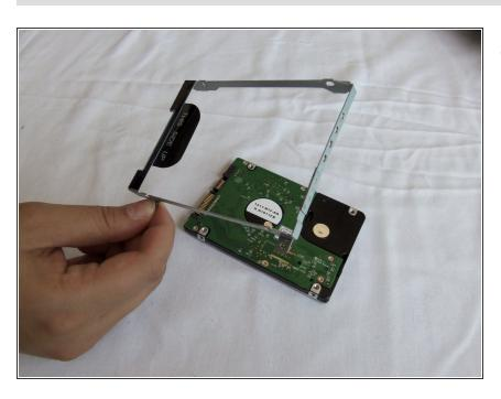
Remove the hard drive casing.
