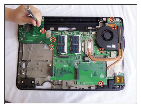
Unscrew the seven 4mm screws with a Phillips screwdriver.
