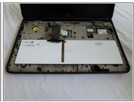
Using the plastic opening tool, slightly lift and rotate the keyboard until it's upside down from the display side of the laptop.
