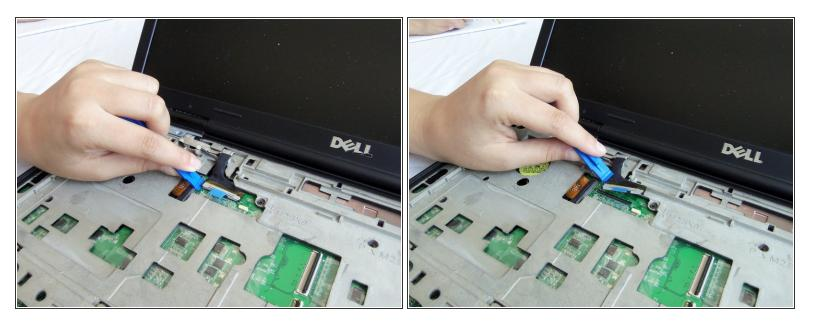
• Using the plastic opening tool, detach the connection from the cable to the board.
