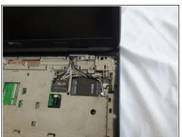
Gently remove the wires for the WLAN and WWAN cards from their housing.
