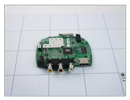
Remove the board from the plastic enclosure and put the board into the replacement enclosure.
