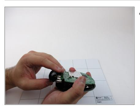
Remove the cover over the A/V ports on the front of the device.
