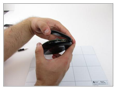
Remove the middle component that is held in place by the top and bottom of the device.
