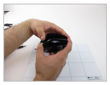
Gently remove the under side of the device.
