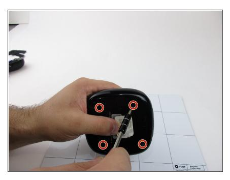
Use the 000 phillips to remove the screws found under all four of the rubber pads.
