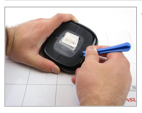
Gently use the plastic opening tool to pry the rubber pads off.
