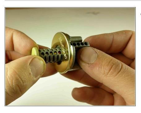
Remove the plug from the cylinder assembly in the upright position so the bottom pins do not fall out.
