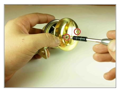
Remove the mounting screws from the thumb-turn side of the lock assembly using a Phillips screwdriver.
