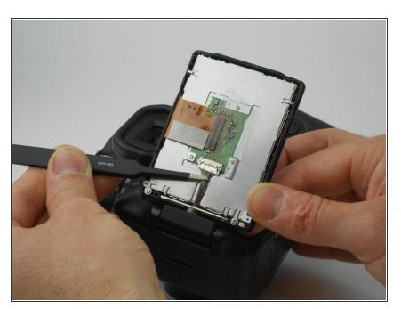
Using the tweezers, carefully disconnect the rear connector by pulling it away from the screen.
