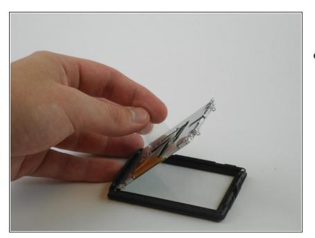
Finally, remove the LCD screen by grabbing the clear plastic tab and lifting it carefully.
