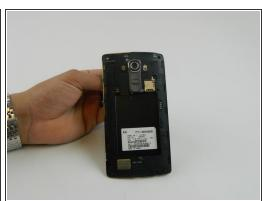
• Remove the **eleven** 3.9 mm Phillips #00 screws found at the back of the phone.
