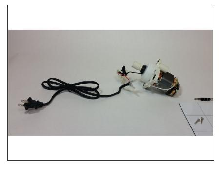
Remove the motor from the motor mounting plate. Pull the motor and cord to the side.
