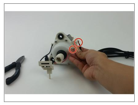
Untwist the brown and the silver wire by gripping the tip and unwinding them. Do the same for the second wire.
