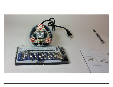
Remove the highlighted screws shown with a Phillips #2 Screwdriver.
