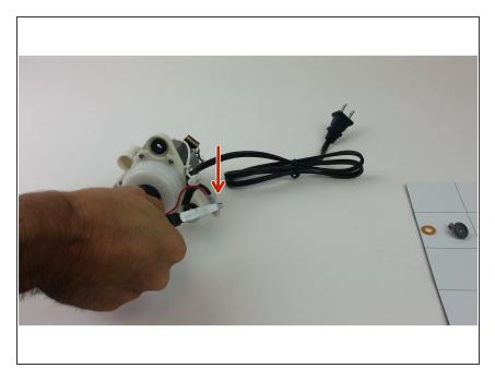
Open the crimp by pressing it opposite to how the crimp was pressed. Repeat for second crimp.
