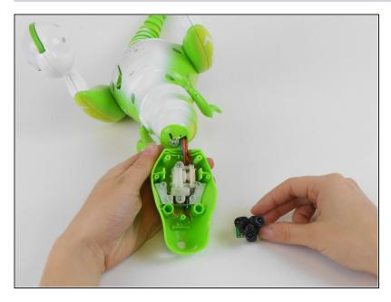
• Remove and replace the nose sensor.
