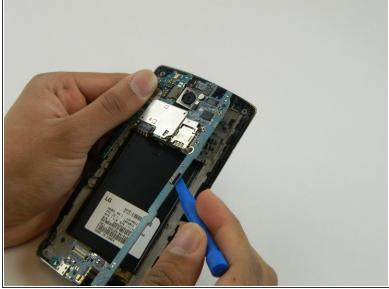
$_{\bullet}$  Remove the motherboard by lifting it up using the plastic opening tool and your fingers .
