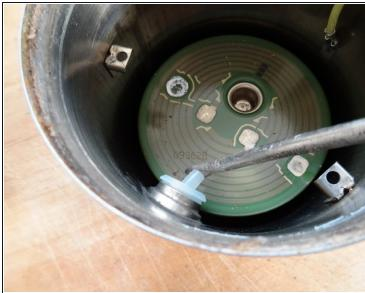
Pull out the circuit board and the motor. After module is removed the on/off pad must be pressed in/through
