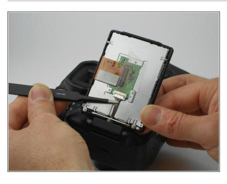
Using the tweezers, carefully disconnect the rear connector by pulling it away from the screen. To reassemble your device, follow these instructions in reverse order.
