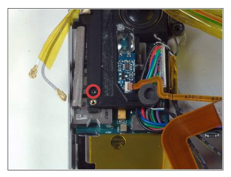
Remove the single black T6 Torx screw securing the left speaker.
