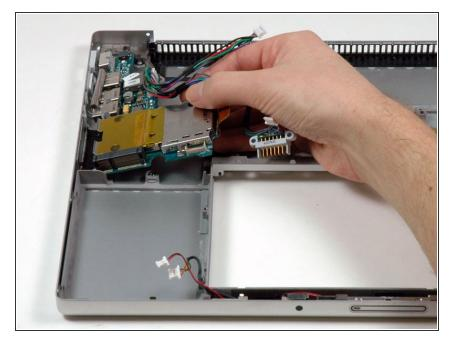
Lift the left I/O board up from the right side and slide it out of the computer.
