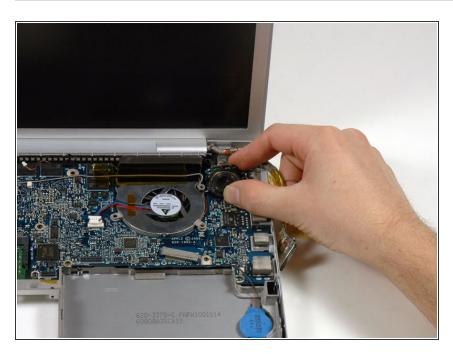
Rotate the speaker clockwise approximately 30 degrees until it comes free from the logic board.
