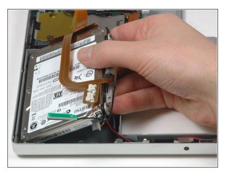
Lift the hard drive and retaining bracket up from the right side and remove it and the attached cable from the computer.
