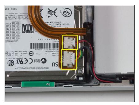
Disconnect the IR and sleep light cables from their connectors above the hard drive.
