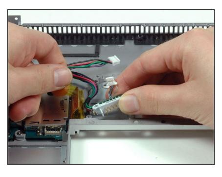
Peel up the orange tape securing the battery connector to the lower case.
