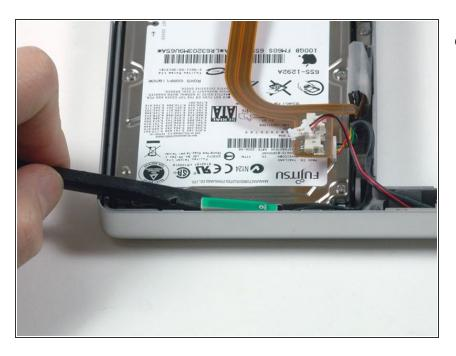
Use a spudger to pry the Bluetooth antenna up from its housing in front of the hard drive.
