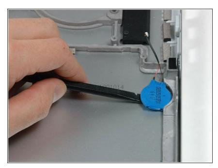
Use a spudger to pry up the PRAM battery off the lower case.
