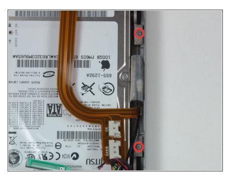
Remove the two silver Phillips screws securing the hard drive retaining bracket to the lower case.
