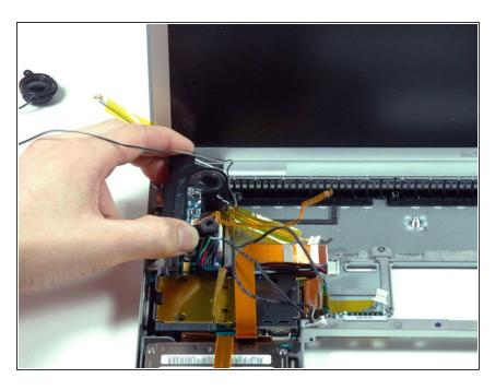
Lift the speaker assembly out of the computer.
