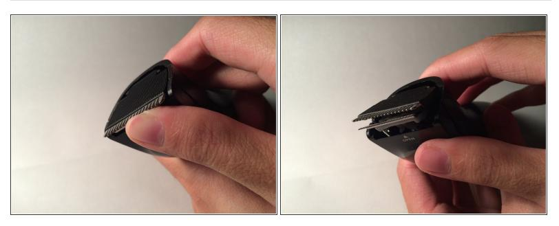
• Place your thumb underneath the blade and push upward to remove it.
