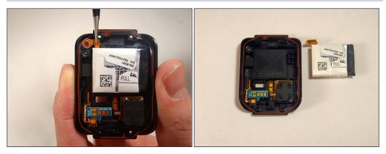
Use a pair of <u>tweezers</u> to peel the battery ribbon cable off of the back cover.
