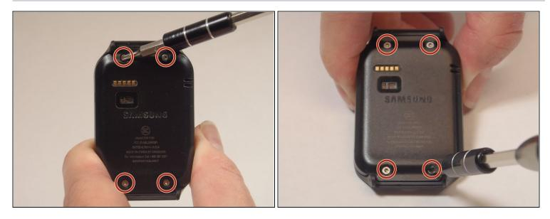
• Use a T5 Torx Screwdriver to remove the 4 (0.4 mm) screws located on the back of the watch.
