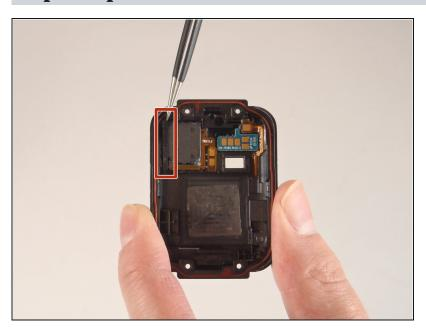
Use a pair of <u>tweezers</u> to remove the rubber gasket. It should come off with ease.
