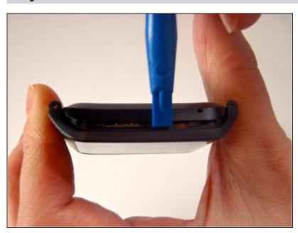
Slide the opening tool in between the two halves of the case and slide along the edge of the watch while gently prying the back cover away from the face of the watch.
