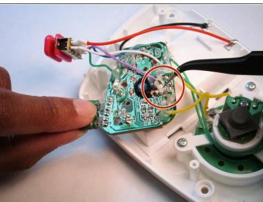
Carefully pull the LED lights off with a pair of tweezers. Once off, put in and connect a replacement.
