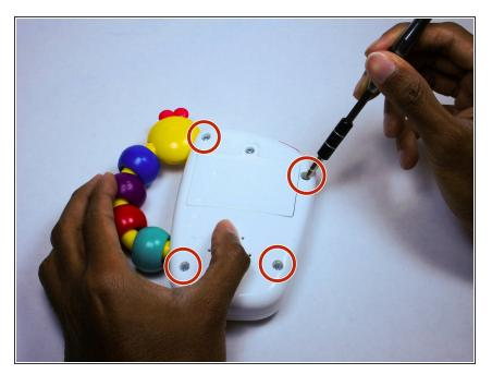
Using a screwdriver loosen the four screws connecting the body of the device together.
