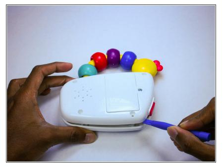
Once unscrewed, pop the back of the device off using the plastic opening tool.
