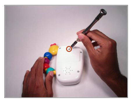
Using Philips #1 Screwdriver loosen the 5mm Philips screw on the battery plate.
