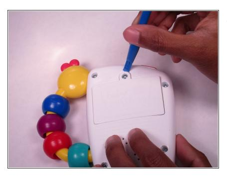
Lift the back with the plastic opening tool.
