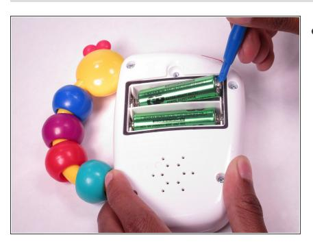
Using your fingers or a plastic opening tool, remove the batteries and replace them.
