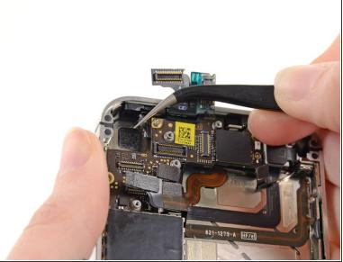
(i) If present, remove the piece of tape covering a Phillips screw near the power button.
