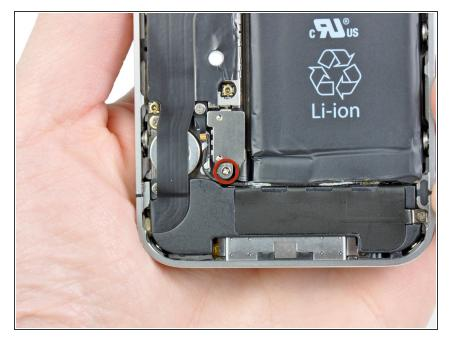
Remove the single 1.5 mm Phillips screw securing the battery connector to the logic board (if present).
