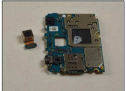
• Grasp the cable with the <u>tweezers</u> and gently pull up and away from the motherboard to disconnect it.
