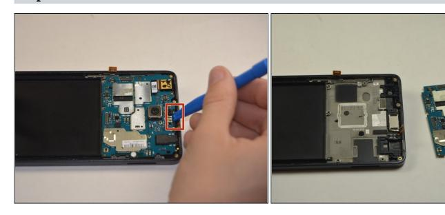
Wedge the plastic opening tool, between the motherboard and the inner region of the phone in the slot atop the motherboard.
