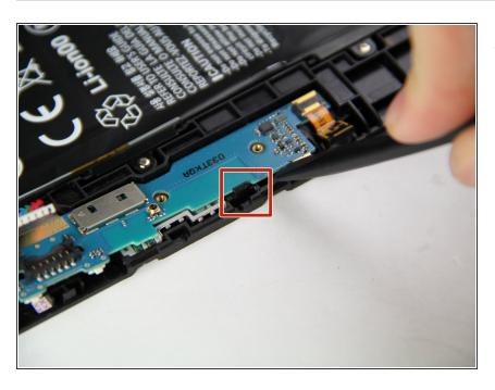
Once the corner is removed, repeat the same action at the far end of the motherboard to release the second clip.
