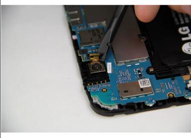
Using the spudger, pry up the connector on the motherboard from the back camera to disconnect it.
