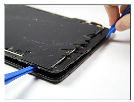
Insert another plastic opening tool (or a similar tool) between the screen and the back panel on the opposite side of the device to hold it open.
