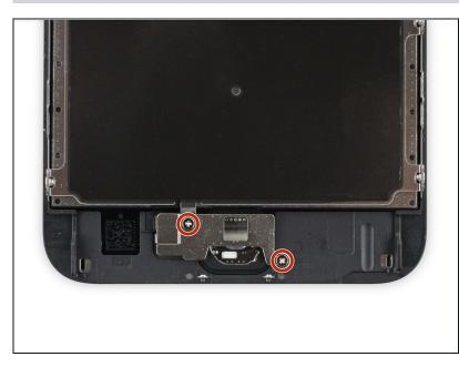
• Remove the two 1.9 mm Phillips screws securing the home button bracket.
