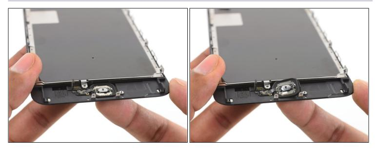
A The rubber gasket surrounding the home button is very thin and tears easily.
