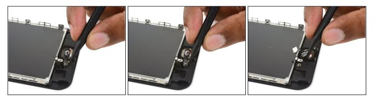
• Use the pointed end of a spudger to pry the lightly-adhered home button flex cable off the display assembly.
