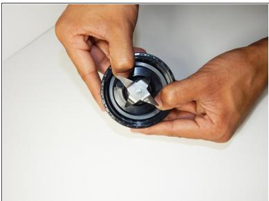
Place and press the new seal into seal seat with finger.
