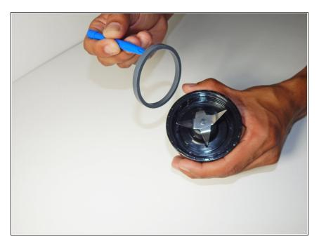
Gently pry the seal up while lifting seal out of the seal seat.
