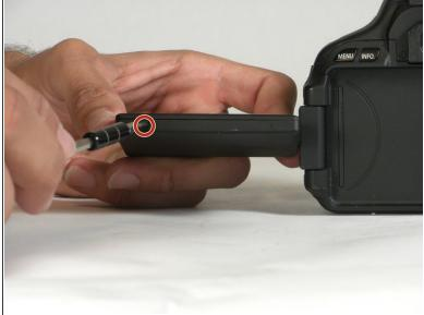
Remove the two 3 mm Phillips #000 screws. The screws are on opposite sides of the screen.
