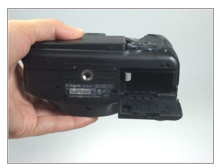
Remove the battery from the compartment.
