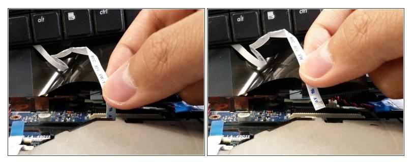
Pull the white ribbon cable out of its slot.
