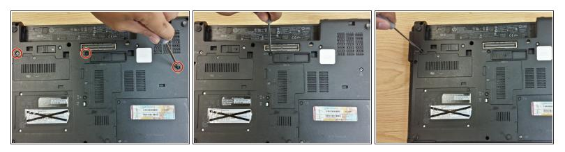
• With a Phillips-head screwdriver, unscrew the three screws marked with the keyboard icon.
