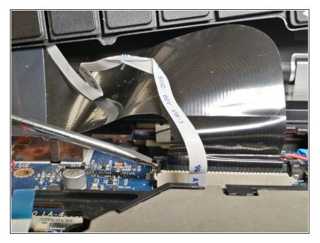
Using a spudger or flat-head screwdriver, pull up the tabs at the black ribbon cable's sides to unlock the cable.
