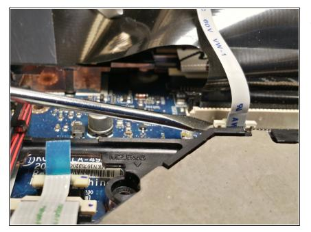
Using a spudger or flat-head screwdriver, pull up the tabs at the white ribbon cable's sides to unlock the cable.
