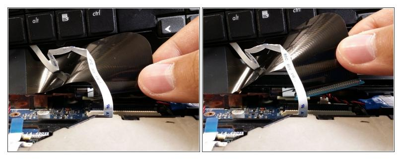
Pull the black ribbon cable out of its slot.
