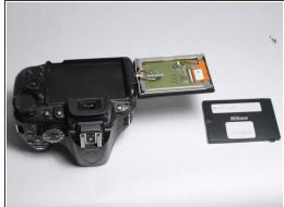
Pry open the plastic casing using the opening tool or by hand.
