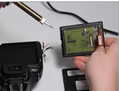
Desolder the three small wires on the left side of the circuit board.
