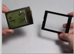
Using a spudger, remove the display from its casing.
