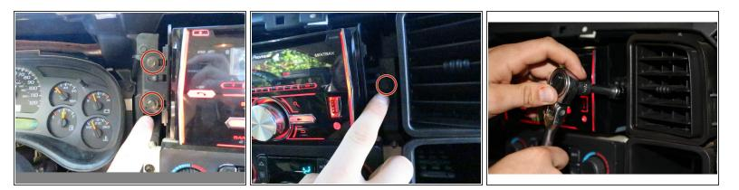
• Remove three bolts using a 7mm socket wrench, two on the left and one on the right.
