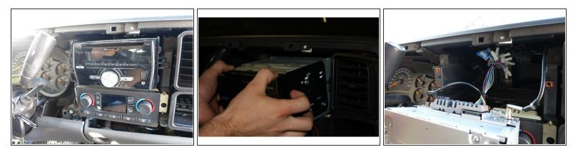
• Remove the head unit once the bolts have been taken out.
