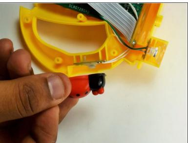
Locate the ladybug button on the handle of the opened flashlight and remove it from its slot.
