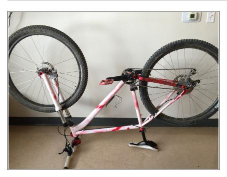
Flip the bike so that it is resting on the handle bars and seat.
