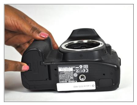
Find the marked arrow on the battery compartment cover labeled "BATT. OPEN". Slide the lever following the arrow's direction and lift at the same time to release the latch.
