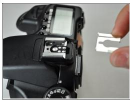
Use a metal spudger or opening tool to gently lift the hotshoe plate and slide it off.
