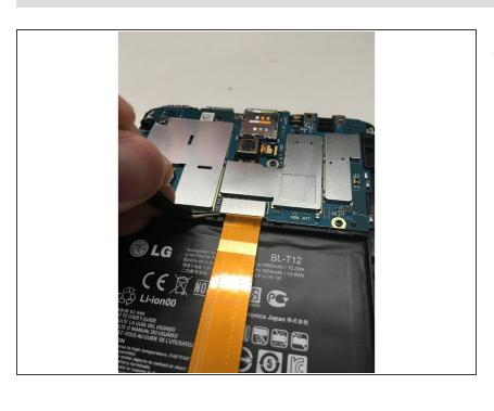
Carefully pry up the charging port connection from the bottom left with your <u>Tweezers</u>.
