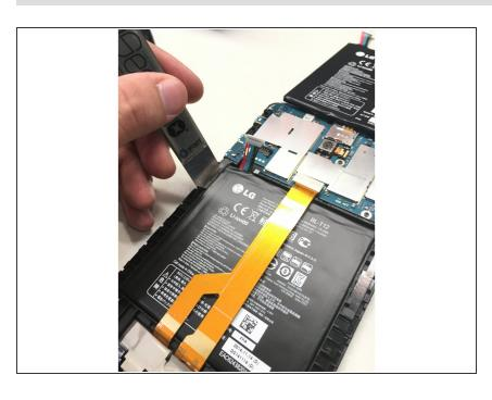
Grab your <u>iSesamo Opening Tool</u> and break the adhesive around the edges of the battery.
