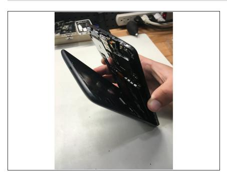
Vuala! We're in! Carefully slide the screen assembly away from the back cover.
