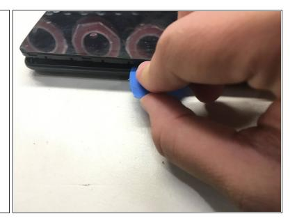
• First things first, use the handy pick iFixit sells on their online store. Carefully pry the frame apart in between the screen assembly an back cover. Be extremely careful, you don't want to damage the motherboard..
