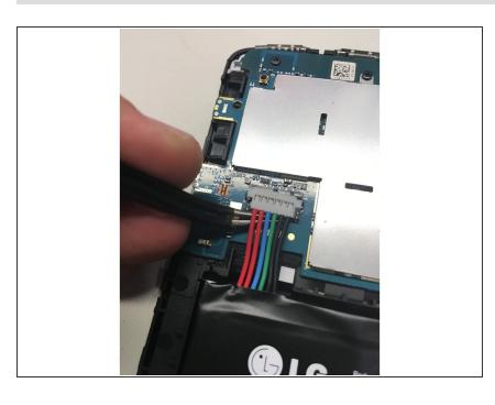
Carefully lift the battery connector.
