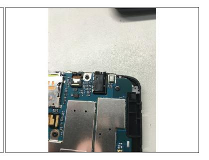
After reconnecting the new battery and charging flex cable, make sure you put the headphone jack back into place.
