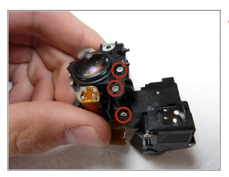
Remove the three screws shown to separate the lens from the viewfinder.
