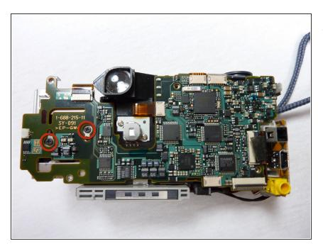
• Remove the two additional screws on the back of the lens.
