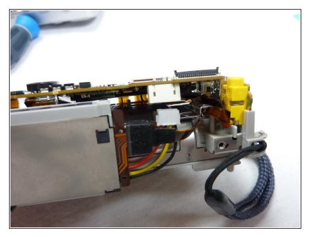
Detach the ribbon cables and unplug the cable leading to the back of the motherboard.
