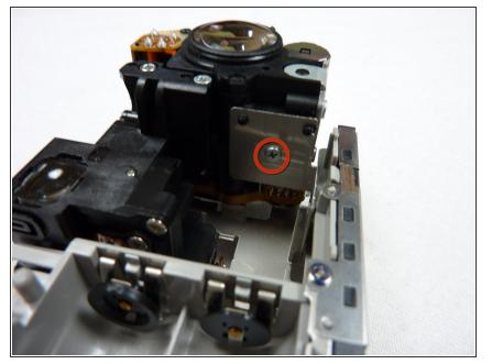
Remove the screw indicated in the picture to detach the lens and the viewfinder from the other hardware.
