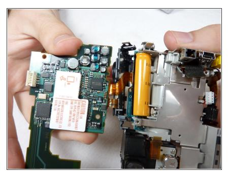
• Remove the motherboard and the flash from the rest of the hardware.
