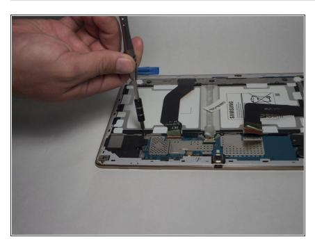
Remove the six 2mm screws Phillips #000 screws surrounding the battery.
