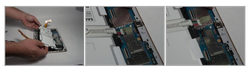
Hold the battery and disconnect the plug to remove the battery.
