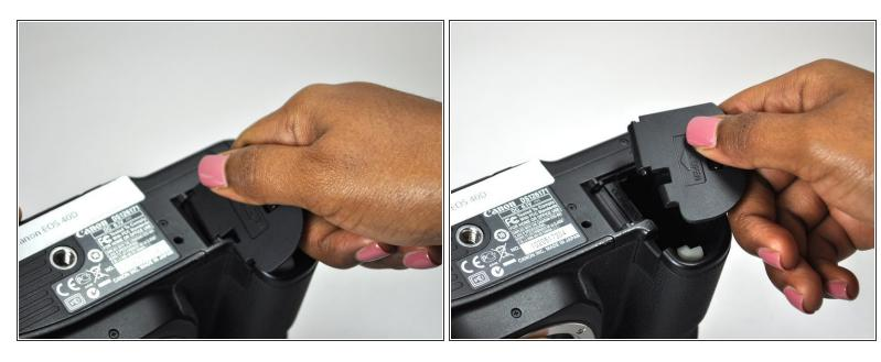
With your thumb, gently press down on the battery door and rotate the battery door clockwise. The upper hinge will pop out and then the lower hinge will pop out.
