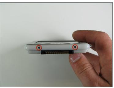
• Remove the four 2.6 mm Philips screws on the top and bottom of the frame.
